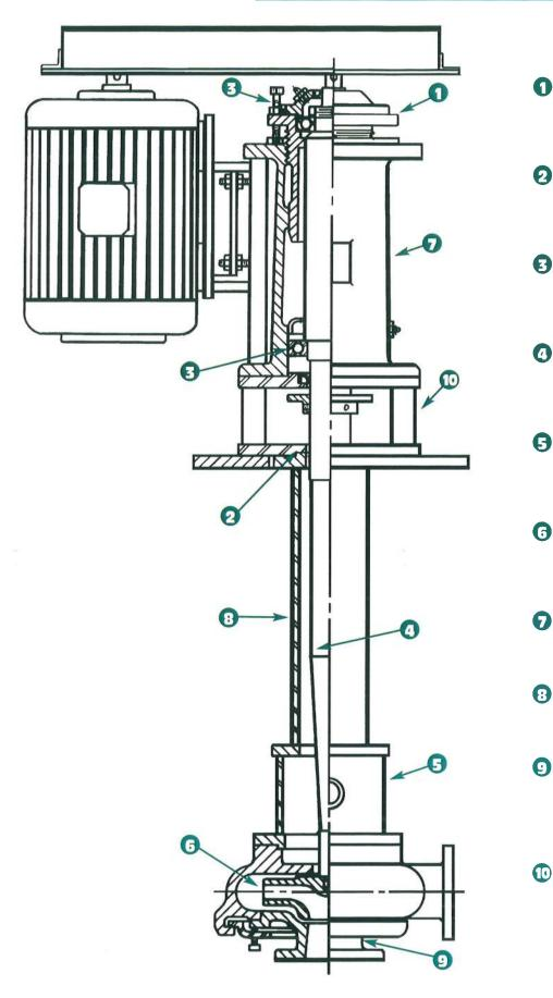
Threaded housing minimizes misalignment and provides precision axial impeller adjustment for maximum wet end wear life
