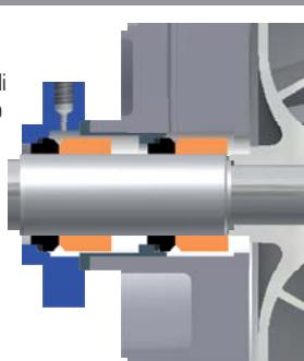
**EN** double tandem mechanical seal. PLAN 52. Also suitable washing connection for the pump side seal.
