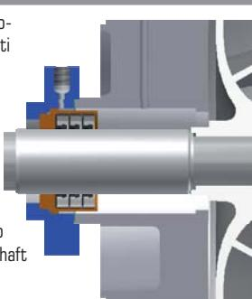
**EN** self-lubricated seal rings suitable for clean and viscous liquids. Also suitable on ceramized shaft sleeve.
