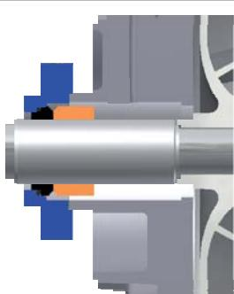
**EN** Self lubricated single mechanical seal
