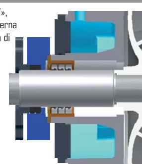
**EN** as «V» type, but with safety gland packing quench and heating chamber.
