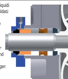
**EN** To use with hot or over-heated liquids and in combination with external heat exchanger. PLAN 23
