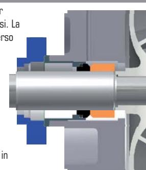
**EN** Single seal for dirty or viscous liquids. Its position, close to the impeller, facilitates lubrication in difficult situations
