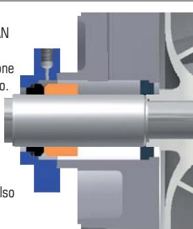
**EN** To use combined with PLAN 11 from the discharge or PLAN 32 from external circuit. Also suitable «E» execution without bottom ring.
