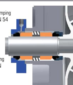
**EN** double back to back seal with pumping ring. PLAN 53 - PLAN 54
