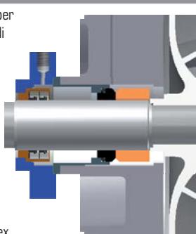
**EN** combined seal, for dry running without auxiliary liquids or for discontinuous flushing. Safety barrier for hazardous liquids or Atex
