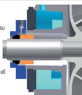
**EN** The heating or cooling chamber can be easily installed on all RD-RG pumps
