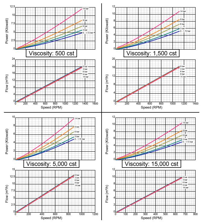
**Standard Clearance Iron Construction** 2" Std. Port Size
