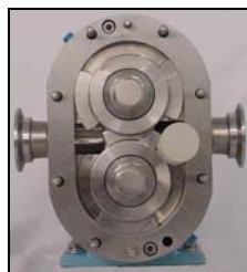
Figure 70 - Tightening Bottom Rotor
