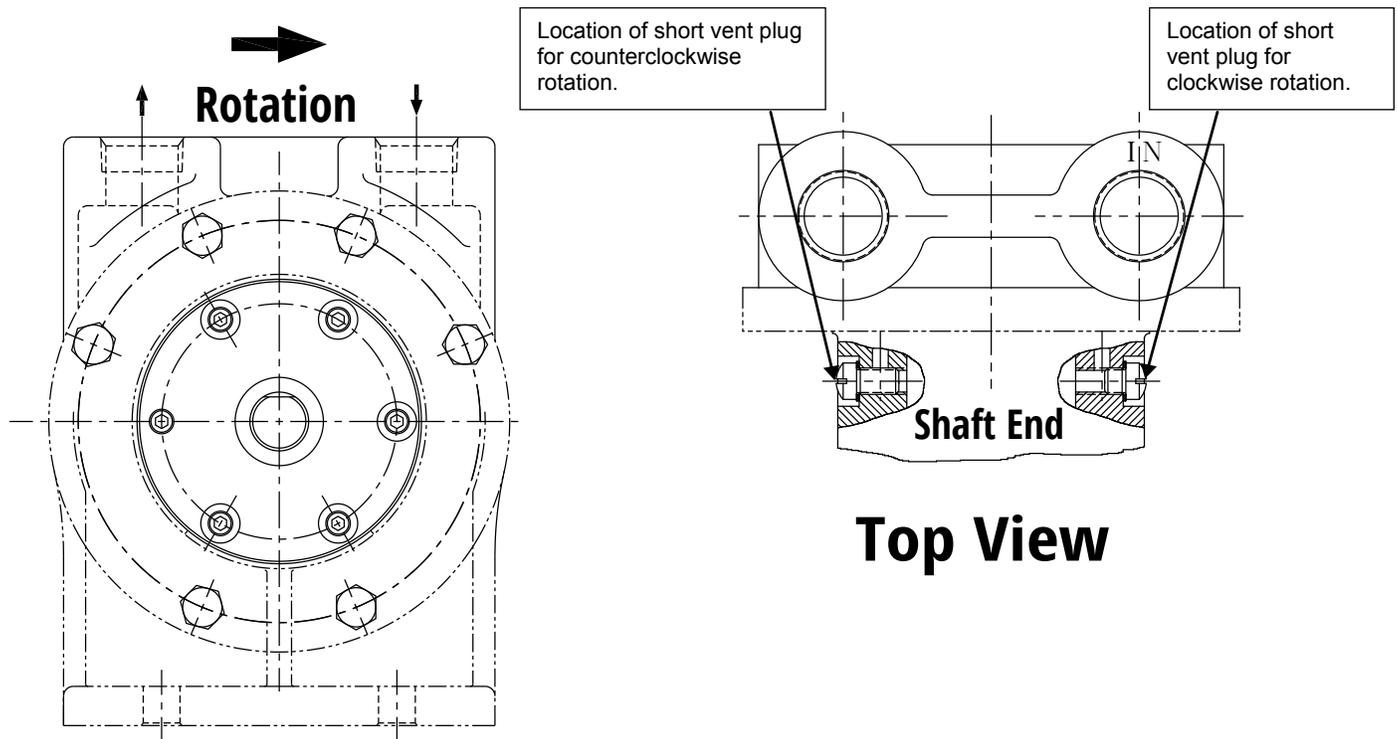
If outfitted with an internal relief valve (model CK1BV), the rotation cannot be changed in the field unless the cover/valve assembly is also replaced. To change the location of the suction port on pumps supplied with Tuthill's unique automatic reversing feature (model RCK1B), the following must be done in addition to the steps above.
